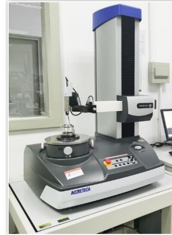
Roundness Measuring Instrument
